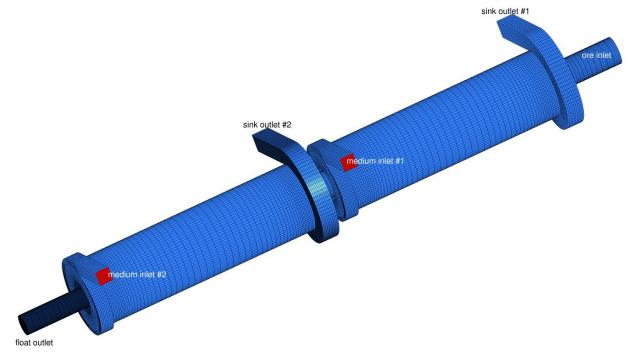
Figure 2 Block structured hexahedral mesh of the considered geometry
