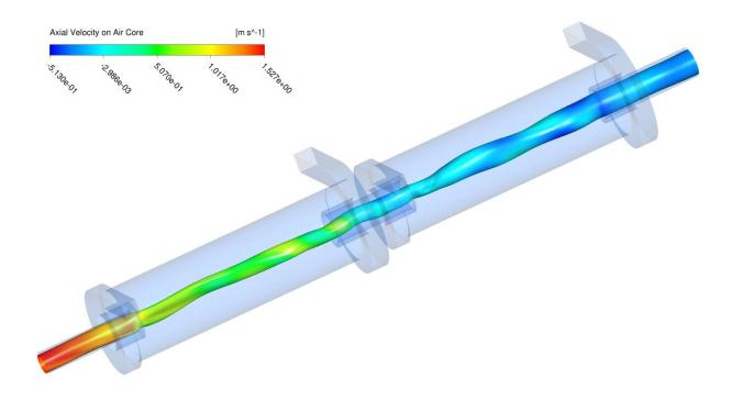
Figure 3 Computed air core colored by axial velocity
