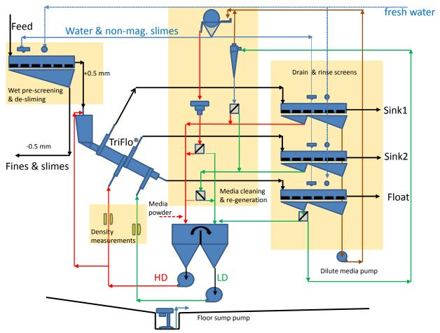
Figure 1 Simplified dense media separation flowsheet with a two cut density Tri-Flo<sup>™</sup> device.
