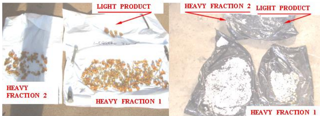
Figure 2. Tracers Separation. Left: 24% Pb crystals; Right: 4 mm Al 2 O 3 particles.
